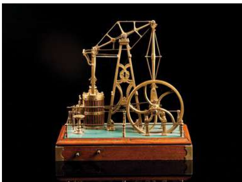
Model of a Walking Beam Steam Engine
