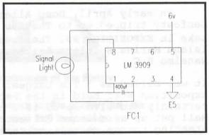
The two Flashing Circuits, although using the same integrated circuit, are slightly different is layout. FC1 is connected directly to the 6 volt source, while FC2 is connected to V<sub>out</sub> of the 2 volt VR. Pin 4 of FC1 is connected to the Expander.
