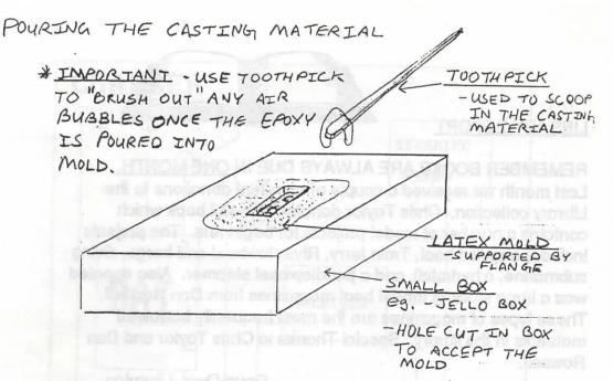
CASTING MATERIAL, IN THIS CASE 30 MIN EPOXY FROM INDUSTRIAL FORMULATORS, WAS USED. THIS EPOXY CAN BE POURED IN FOR A LARGE MOLD OR SCOOPED IN FOR A SMALL MOLD.
