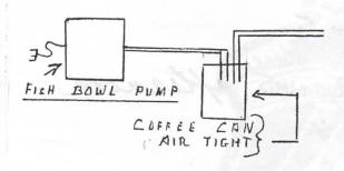
A small fish bowl pump can supply adequate supply of air for torch, instead of blowing into the torch. The can supplies a steady supply of air. Without this a pulsating effect from the pump might happen. The coffee can must be air tight and stand a small pressure. Don MacLeod
