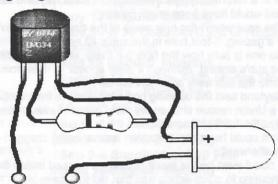
Please note that the markings on your chip may well be different than that shown above. It should say LM334Z on it somewhere though. Make sure if you are asking for (or ordering) it by name to add the Z on the end, as the other versions are too big for most model use. The Z version is the most common and commercially available version.
