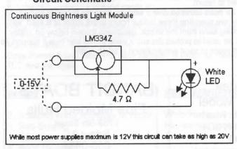
Wiring the circuit could not be easier. As there are only two components (three if you count the LED), there is no need for circuit boards. Simply solder the components together in a shape that suits your available space. Please note the orientation of the chip, as it must be wired one way only. The LED must be wired the correct way around too. Note the following points to identify the correct polarity:
