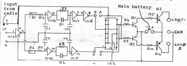
The circuit requires that you connect a power battery at the point shown because this device can switch heavier current loads than the receiver battery can supply. This extra battery can be the same one that you run your motors from.
