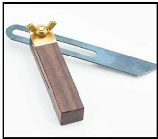
These two items have been in my tool box for some time and have really been an asset in building. The Strip Cutter above, cuts wood or plastic up too 1/4" x 1/4" or 1/8" x 1/2". Really handy on hull construction. I purchased mine at Michael's. The sliding bevel square is only 3" in length and I have found it a really handy tool for building superstructures or cabins on my models. It's another low priced item from Lee Valley.
