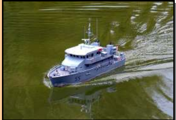
Bow and stern waves demonstrated by Alex James’ superb rendition of the CF’s new Orca 55 . The full-sized Orca Class Patrol Craft Training vessel measures 33-metres long, with a displacement of 210 tonnes and a top speed of 20 knots. Photo by Bill Sturrock.
