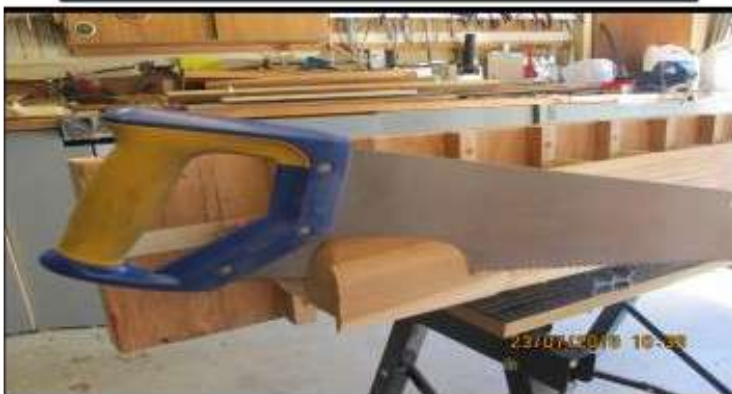
Below shows cutting off a piece of waste at the stern to create stern bottom. The hand saw seemed easier than doing a lot of planning
