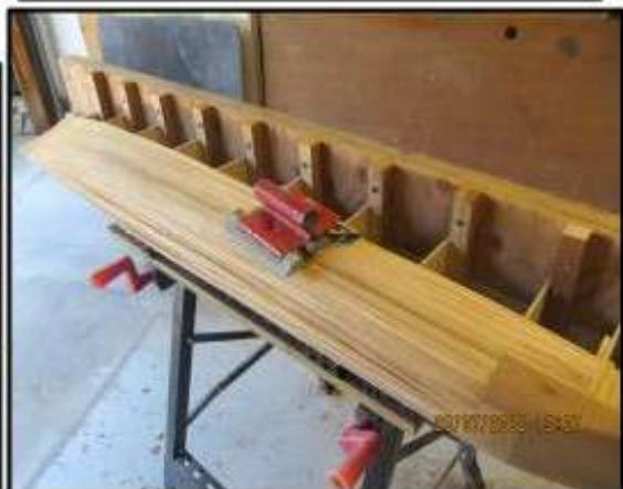
Final sanding getting ready for nylon covering and polyurethane coating.
