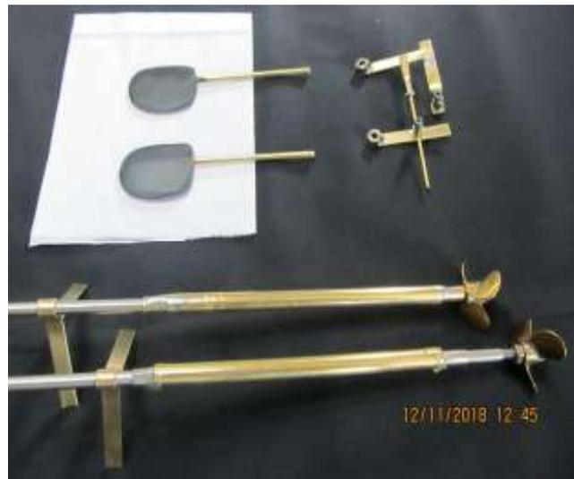
Gluing the deck down with Tight Bond Green glue, the product used throughout the wood construction. The next shows the rudders, steering arm . The shafts are stainless with home made stuffing boxes. Propellers purchased at Burnaby Hobbies during a recent trip to the mainland.
