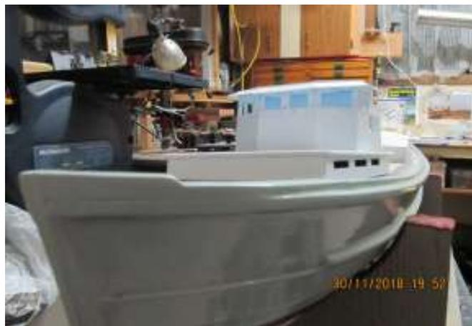
These four pictures show construction of the rear and front deck house as well as the wheel house. All styrene construction from the deck up. The boat is very light at this point in construction just under four pounds. Next is bathtub testing and getting the vessel near it's designed waterline.
