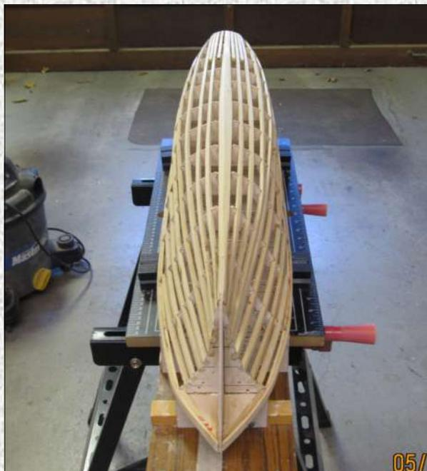
As you can see, the planking is progressing and gunwales are in position. The gunwales are made up of two layers, laminated in position. This made it possible to easily make the sharp bend at the bow. Adhesive is "Tight Bond #3 ". In my mind a excellent product for hull construction.
