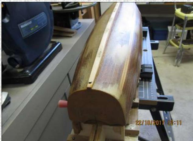
Now the external skeg is mounted by screwing, glue and plugging through to the keelson . Note the screw and washer at the stern.. I use this system as a clamping crew. It's removed when the glue is well dried and plugged. The hull is now ready for a couple of final coats of ploy before conventional undercoat and final finishing.
