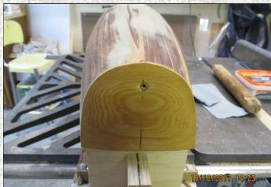
Picture on the left shows all the stringers in position and faired, ready for strip planking. At the bow I will fit red cedar blocks once the planking is finished. These blocks must be very dry and making a purchase of Kiln Dried material such as Bass wood or Red Cedar is the best way to deal with solid bow blocks.
