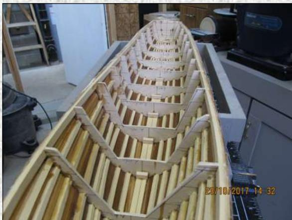
The hull is now removed from building board and cleaned out made ready for motors, radio etc. This hull now weighs 2.5 lbs. I would like to have a finish weight of no more 6 lbs without the battery. I suspecting that I'll have to watch my weight build up carefully.
