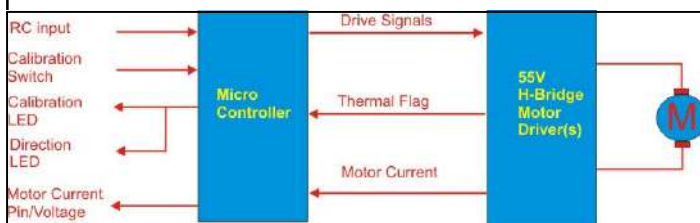
Figure 5: Block diagram of ESC 2010 Speed Controller
