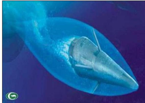
Artist's rendering of the supercavitating missile in its cocoon. Note that not all illustrations show the same longitudinal position of the fins on the body.
