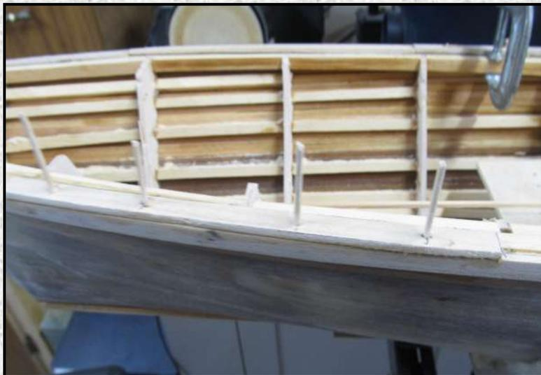
The boat is now off the building board, sanded and made ready for priming at a later date. This picture shows the gunwales on and toe rails in progress. You will notice I am using tooth picks for plugs.
